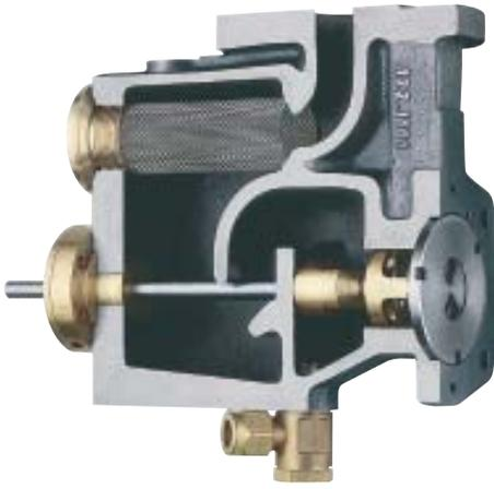
Incoming steam is filtered, dried and drained in the **connection unit** and then fed into the distribution system at the desired rate. The steam passes through the flanged connection which is a standard feature of the system and saves the customer the problem of extra
